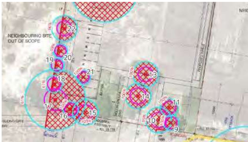
Figure 8. An image of the NRZ calculation for Trees 9-22 with the red hash showing encroachment of proposed build. Civica ArborSafe, March 2026.
